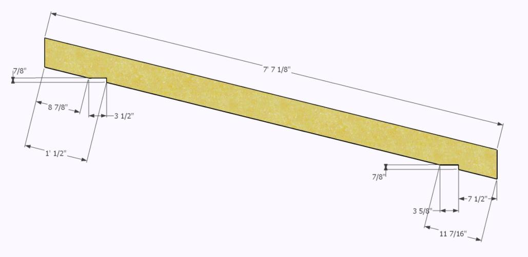
Rafters - you will need 5 of these and two without the notches for the outer rafters
